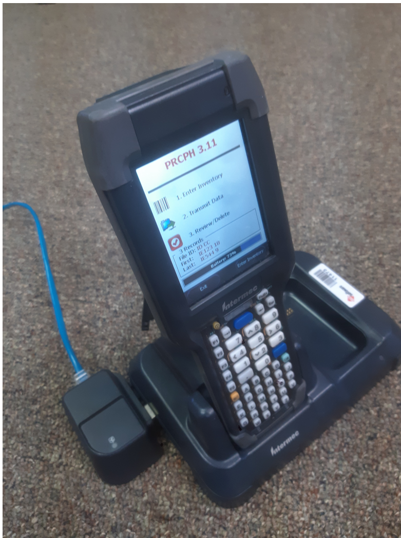
Example of an Ethernet Module Hookup
